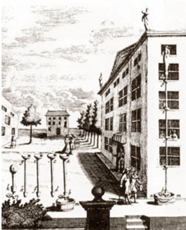
Otto von Guericke's water barometer from 1654. Mercury makes a barometer of a much more manageable height!
